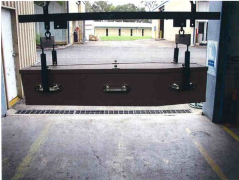
Photo A3. Performing the 30 minute suspension test on the casket with the lid in place after conditioning for 7 days at a temperature 3 \pm 2 C
