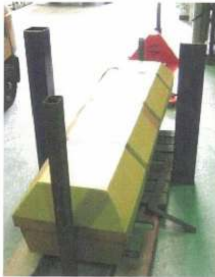
Figure 1. Showing typical test set up with reference posts to measure the distortion under loading.
