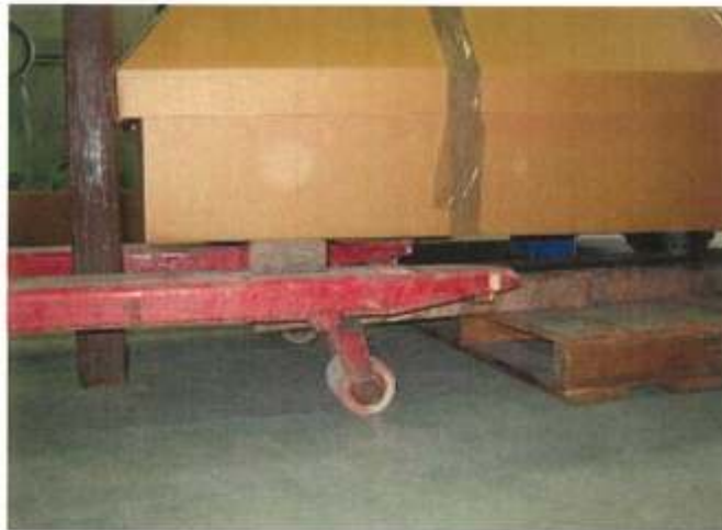
Figure 2. Showing typical test set up with reference to lift points as shown by timber block. Also showing the taped bands.
